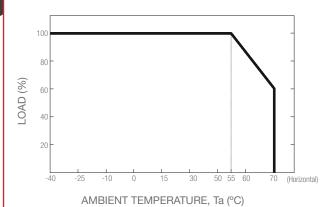
If 39.019 operates in cosntant current mode with the rated current, the maximum workable Ta is 55°C.
